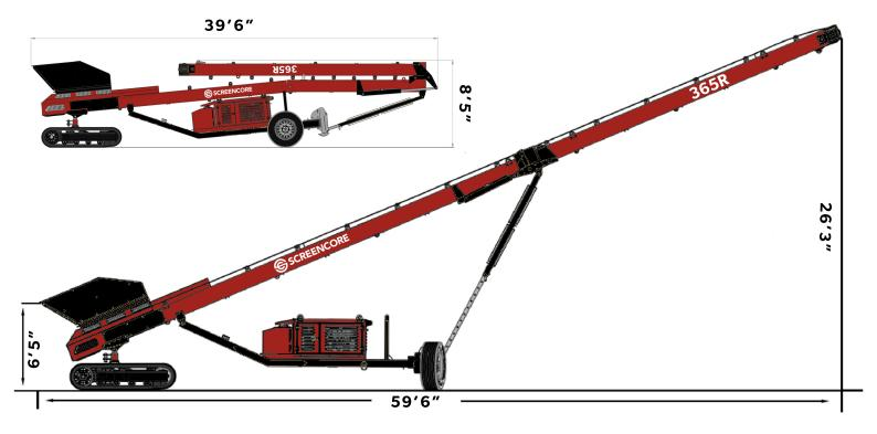
The Screencore 365R is a heavy-duty 65' tracked radial stockpiler giving the operator ultimate flexibility with material movement and placement.
