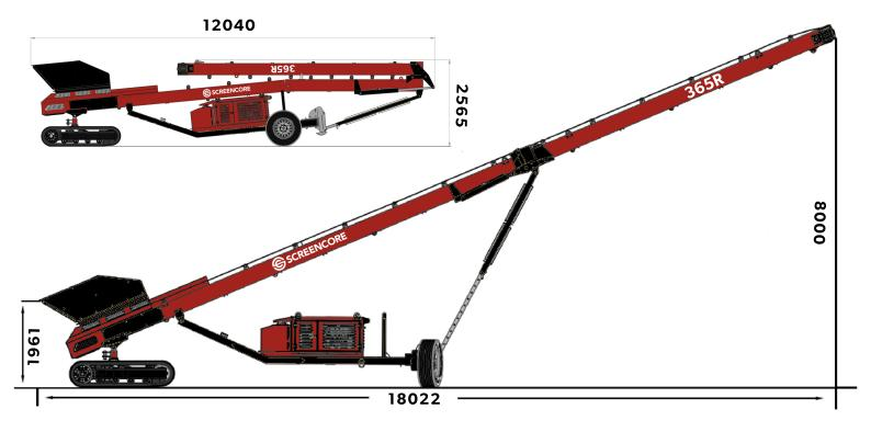
The Screencore 365R is a heavy-duty 19m tracked radial stockpiler giving the operator ultimate flexibility with material movement and placement.
