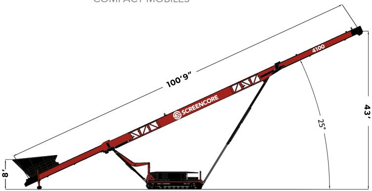
The Screencore 4100 is a 100' heavy-duty stacker with the ability to build a stockpile of over 40' in height at massive production rates
