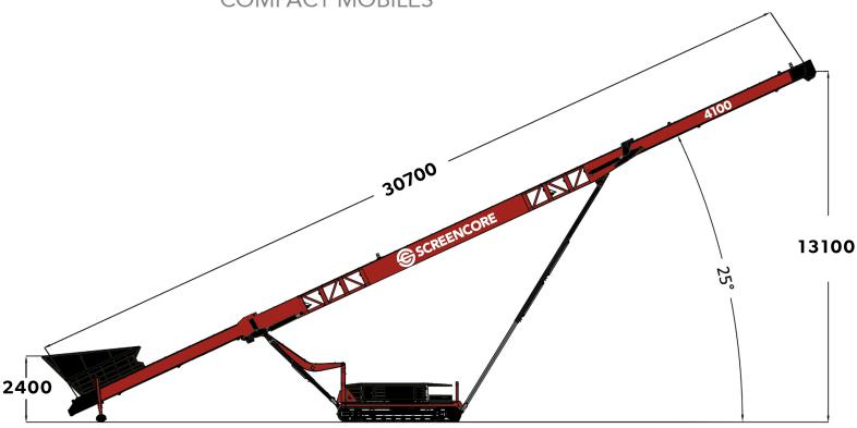
The Screencore 4100 is a 31m heavy-duty stacker with the ability to build a stockpile of over 13m in height at massive production rates
