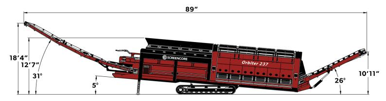
The Orbiter 237 Trommel is a massive screening screening unit for the large operator and creates a radial fines stockpile to optimise screening time and reduce double-handling of fines material.
